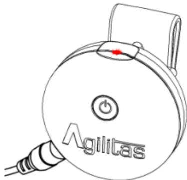
Once the battery is fully charged the red light will **switch off**. A full charge will take approximately **4 to 5 hours**.
