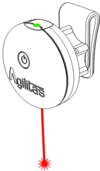
3. To cycle through the sensitivity levels, **double tap** on the side of Agilitas. The next sensitivity level will be activated, and the number of rapid flashes by the green **indicator light** and laser cue will change. Level 1 (1 flash) is the least sensitive and level 6 (6 flashes) is the most sensitive.
